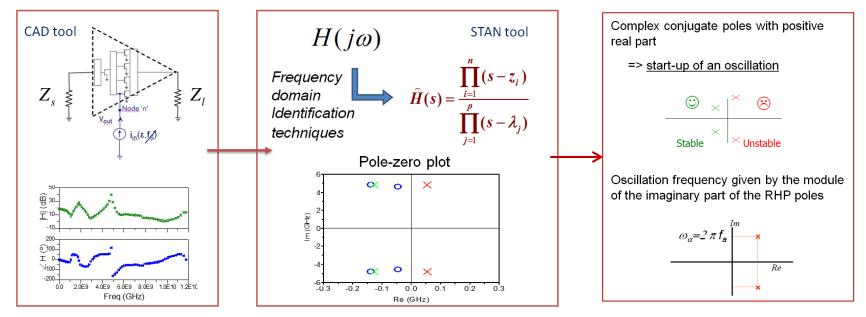
**Pole-zero identification** is a complete stability test. It is able to predict whether a circuit **will or will not** oscillate<sup>1</sup> for fixed source and load terminations  $Z_s(\omega)$  and  $Z_l(\omega)$ .
