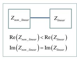
"Exhibiting negative resistance " does not mean necessarily the startup of an oscillation. Having a negative resistance is only half of the story. For oscillation, the fulfillment of a necessary condition on the imaginary part of the impedances is also required. Thus, the criterion is telling us that, due to this negative resistance, the circuit **might** fulfill the oscillation startup conditions once completed with some actual load and source impedances.
