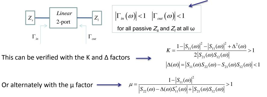
If the circuit is not unconditionally stable, we can trace the stability circles to determine the region of the smith chart for  $Z_I(Z_s)$  that yield  $|\Gamma_{in}(\omega)| > 1$   $(|\Gamma_{out}(\omega)| > 1)$
