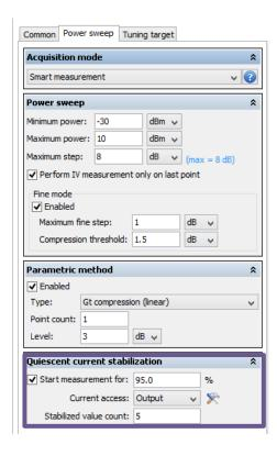
IQ.Star includes a customizable current stabilization feature that allows a recovery time between two power sweeps - Very useful for GaN device based circuits presenting trapping phenomena.
