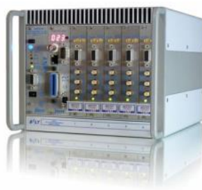
A very small 5-slot BILT chassis hosts the BE2501 and BE2435 modules (photo is not contractual)
